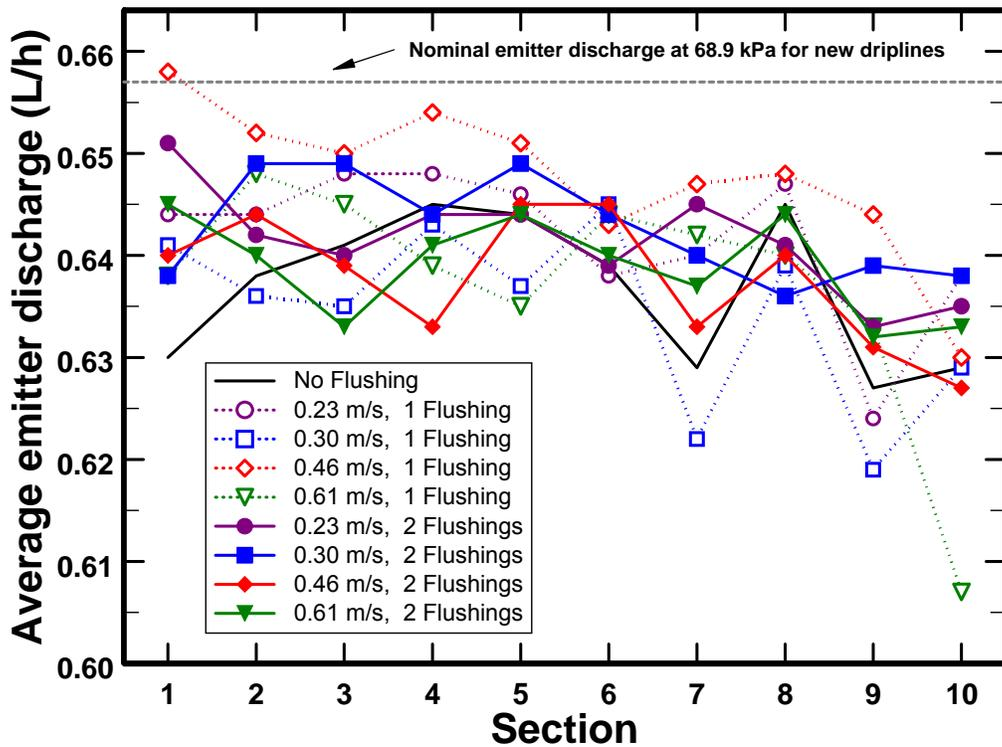
Figure 4. Average emitter discharge for each dripline section as affected by flushing velocity and the number of flushings. Section 1 is at the inlet and section 10 is at the distal end. Note: The average emitter discharge for the dripline sections only vary by less than 8%.
