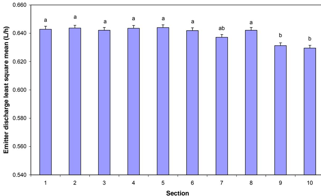
Figure 6. Discharge from the SDI emitters (least square mean  $\pm$  standard error) as affected by section of the dripline (Section 1 is the inlet and Section 10 is the distal end). Different lowercase letters above each column indicate significant differences at  $P < 0.05$ . This data is averaged across all flushing treatments to indicate the effect of location within the dripline on emitter clogging.
