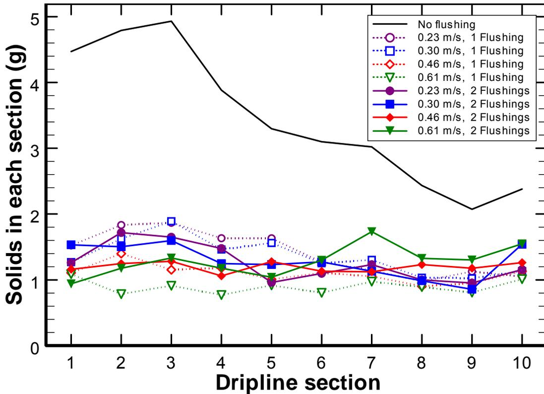
Figure 3. Solids recovered from each dripline section and flushing treatment at the end of the field study. Section 1 is at the inlet and section 10 is at the distal end.
