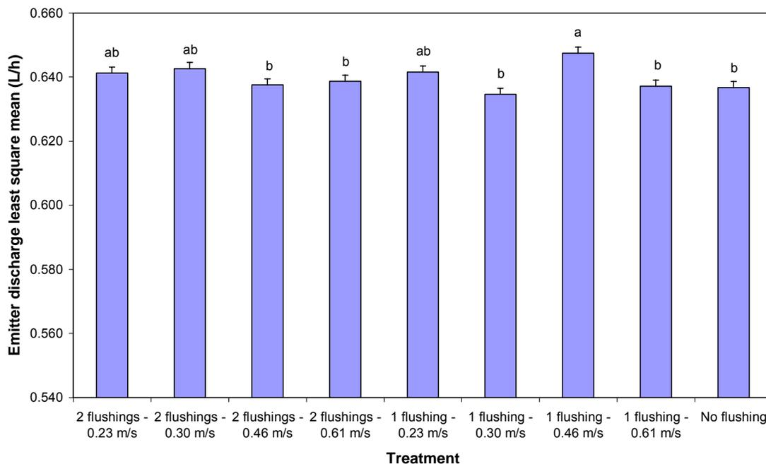
Figure 5. Discharge from the SDI emitters (least square mean  $\pm$  standard error) as affected by flushing frequency and flushing velocity. Different lowercase letters above each column indicate significant differences at  $P < 0.05$ . This data is averaged across all dripline sections to represent the overall effect on the dripline of flushing treatment.
