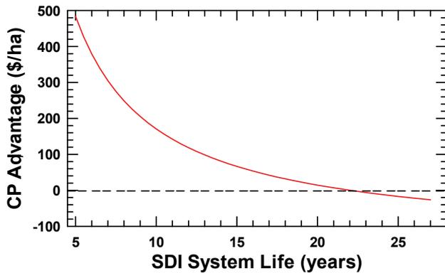
Figure 1. Annual economic advantage of center-pivot sprinkler irrigation over SDI for corn production as affected by the longevity of the SDI system (data from KSU software using 2016 economic assumptions; Lamm et al., 2016).
