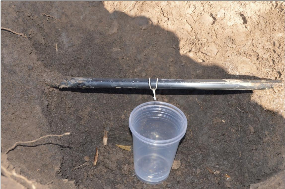
**Figure 2. Arrangement for measuring emitter discharge over a 20 min period.**
