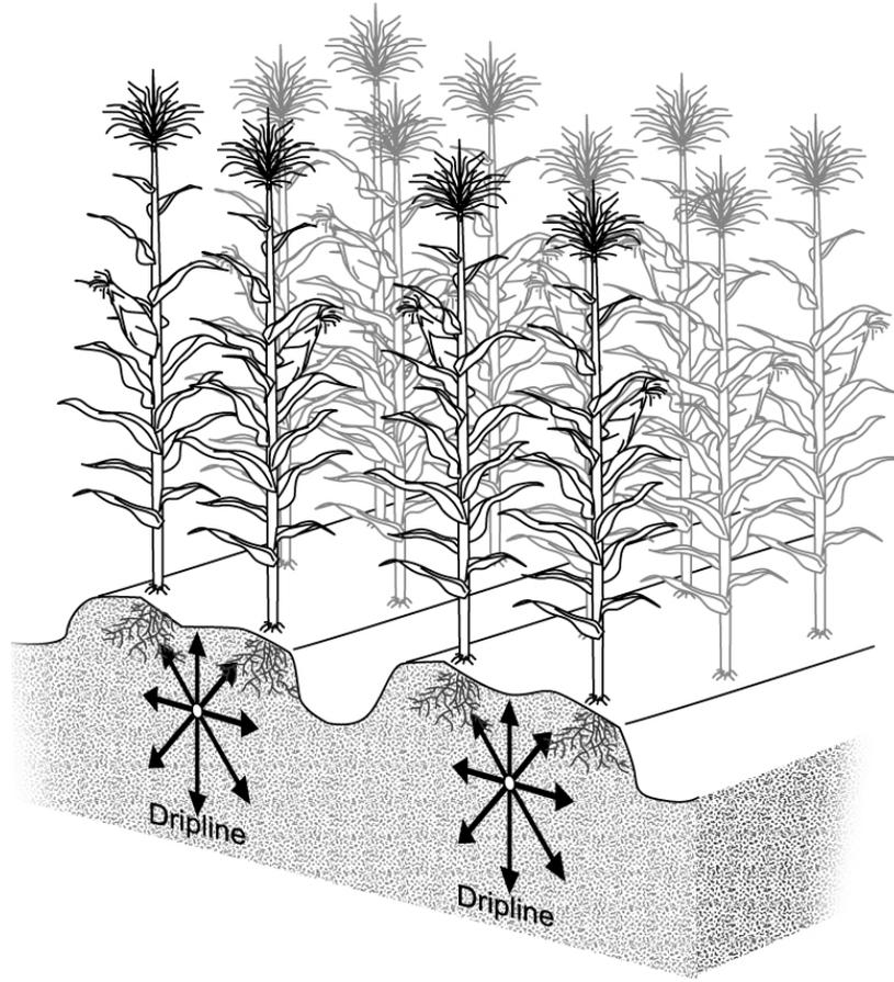
Figure 1. Alternate row/bed 5 ft SDI dripline spacing for corn rows spaced at 2.5 ft. Each plant row is approximately 1.25 ft m from the nearest dripline and has equal opportunity to the applied water.
