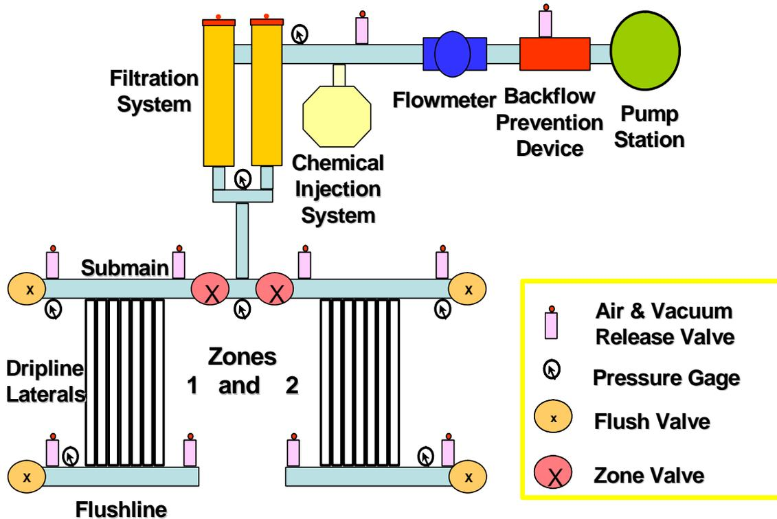
Figure 2. Minimum required components of an SDI system. Components are not to scale. After Rogers, 2003b.
