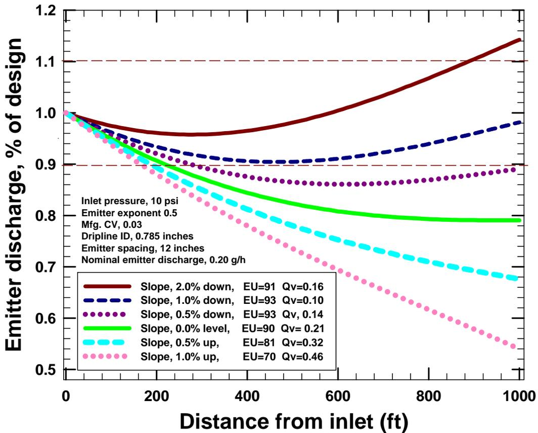
Figure 5. Calculated emitter discharge, emission uniformity (EU), and emitter discharge variation ( $q_{var}$ ) as affected by topography. Results for hypothetical dripline calculated with software from Roberts Irrigation Products (2003).
