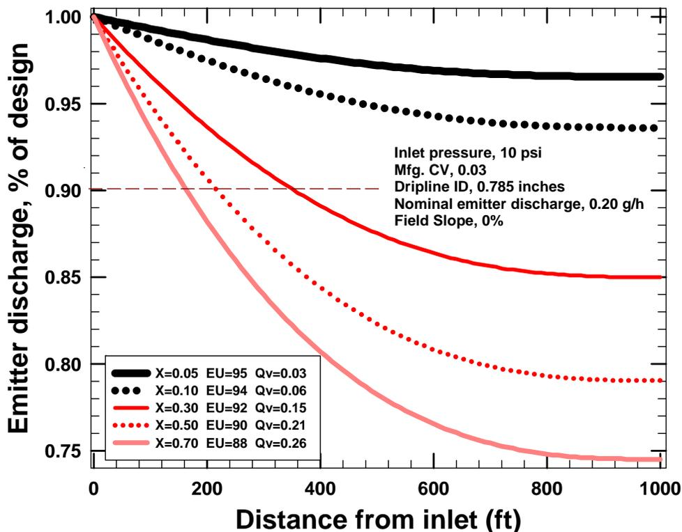
Figure 6. Calculated emitter discharge, emission uniformity (EU), and emitter discharge variation ( $q_{var}$ ) as affected by the emitter exponent ( $x$ ). An emitter with an exponent of zero is said to be fully pressure compensating (PC). Results for hypothetical dripline calculated with software from Roberts Irrigation Products (2003).
