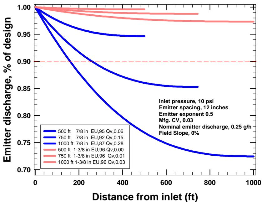
Figure 2. Calculated emitter discharge, emission uniformity (EU), and emitter discharge variation ( $q_{var}$ ) as affected by dripline length and inside diameter. Results for hypothetical dripline calculated with software from Roberts Irrigation Products (2003).
