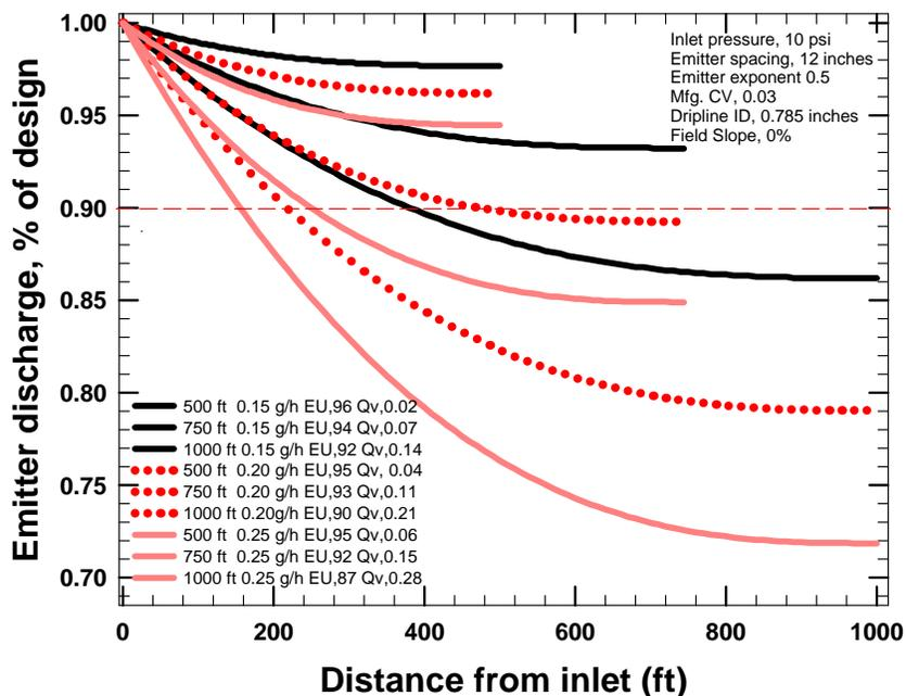
Figure 1. Calculated emitter discharge, emission uniformity (EU), and emitter discharge variation ( $q_{var}$ ) as affected by dripline length and nominal design emitter discharge. Results for hypothetical dripline calculated with software from Roberts Irrigation Products (2003).
