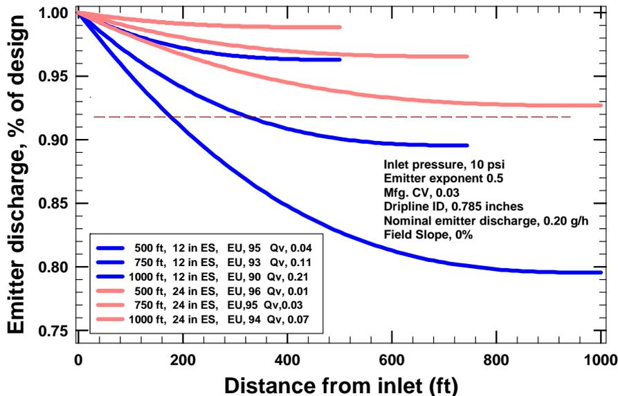
Figure 4. Calculated emitter discharge, emission uniformity (EU), and emitter discharge variation ( $q_{var}$ ) as affected by dripline length and emitter spacing (ES). Results for hypothetical dripline calculated with software from Roberts Irrigation Products (2003).
