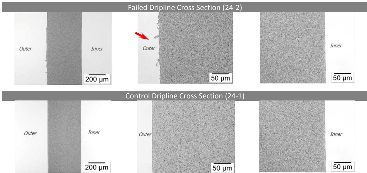
A review of cross section images shown in Figure 7 and Figure 8 indicate remarkable level of carbon black dispersion and homogeneity by today's standards in dripline material used.
