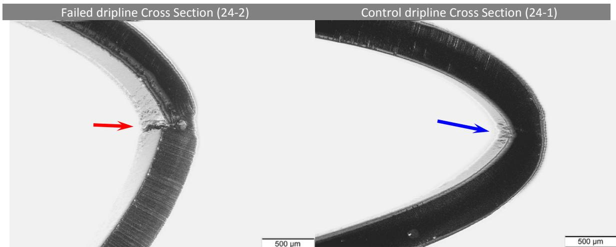
Figure 7 contains higher magnification views of the cross section of the failure region of both the failed and control driplines. Surface striations were present along the inner surface of a control dripline which followed the edge crease (blue arrows). Outer surface deformations
