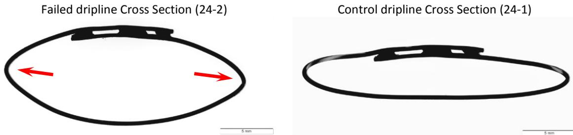
Figure 6 contains dripline cross sectional optical microscopy images taken at the failure region of the dripline. Surface striations were present along the inner surface of a control dripline which followed edge creases (blue arrow). These inner surface striations acted as crack initiation sites for the failures as shown by the internal cracks (red arrows) in the failed in-service dripline.
