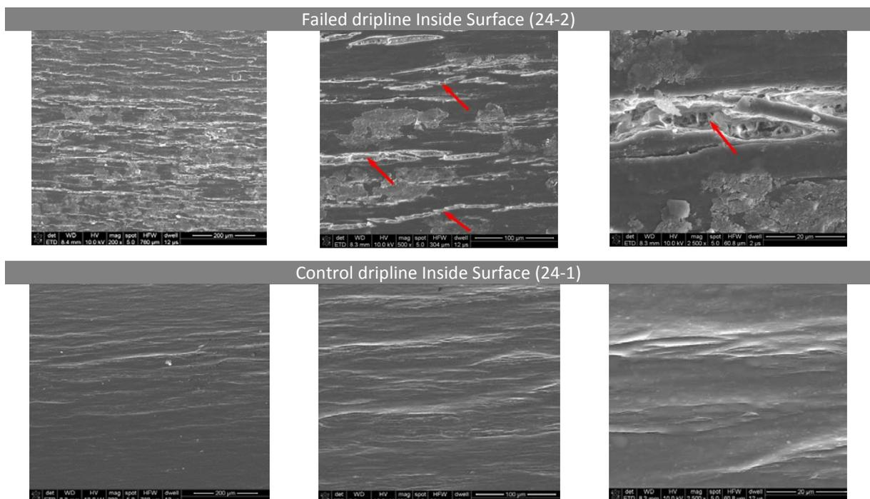
Comparison of the inner surface of the crease region of the dripline using SEM shows the surface striations present in the control driplines, shown in Figure 10 and highlighted with blue arrows. The cracks on the inner surface crease region are also shown in the failed dripline (red arrows), with cracks penetrating approximately 40um into the wall of the dripline.
