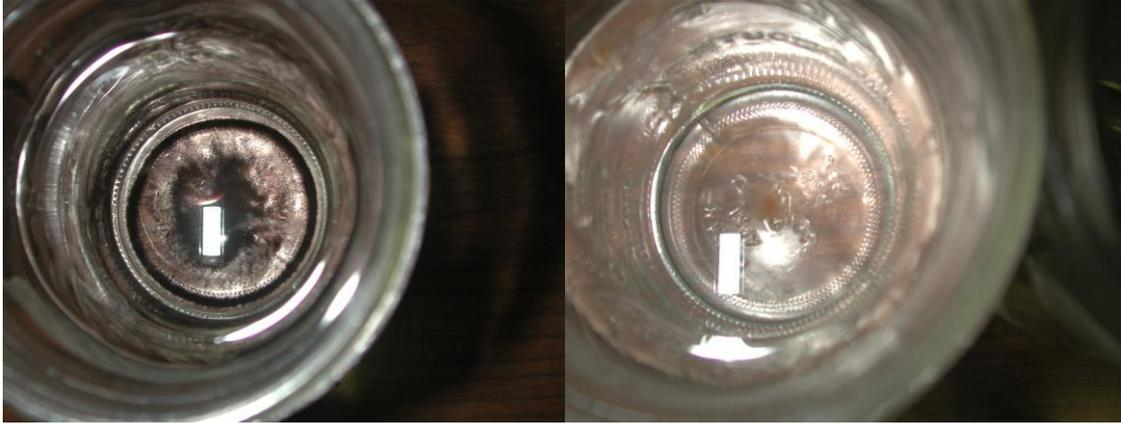
Figure 2. Jars containing Mn at 0.15 g material/gal of irrigation water, both at 0.125% H<sub>2</sub>O<sub>2</sub> concentration. The pH of the container on the left was 7.6; the pH of the container on the right was 6.5.
