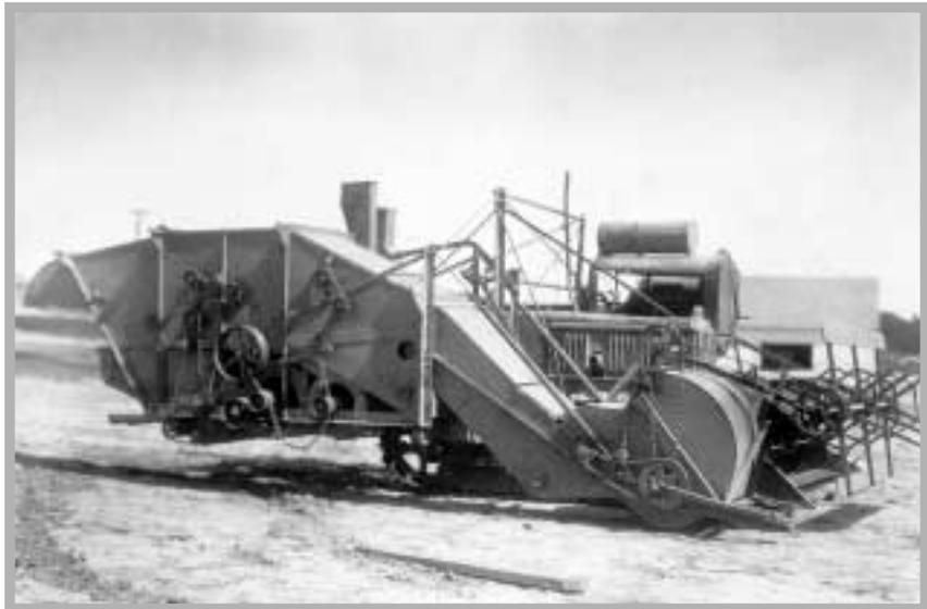
*Combine mounted on Caterpillar tractor for harvesting experimental grain plots. This machine, designed by Aicher, was no doubt the first self-propelled plot combine.*
