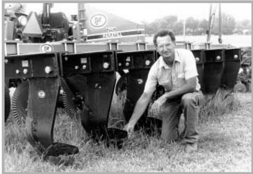
*Carlyle Thompson with a deep tillage tool used to improve water intake into the soil.*
